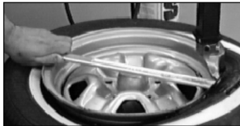
Figure 10 - Lift Bead Over Demount Head
