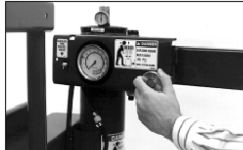
Figure 7 - Adjust Swing Arm to Position Head Roller
