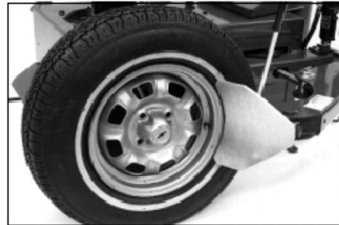
Figure 2 – Position Tire and Bead Loosener Shoe
