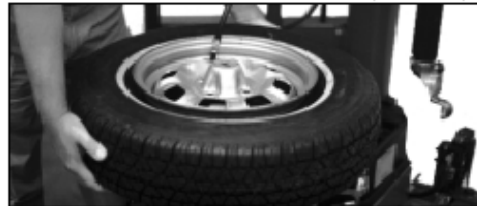
Figure 17 - Lift Tire Upwards for Bead Sealing
