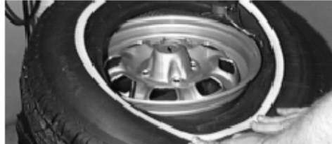
Figure 16 - Mounting Top Bead
