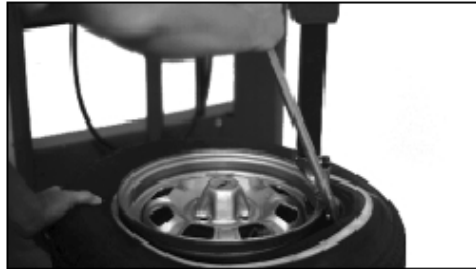
Figure 9 - Insert Bead Lifting Tool
