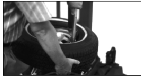
Figure 11 - Demounting Lower Bead
