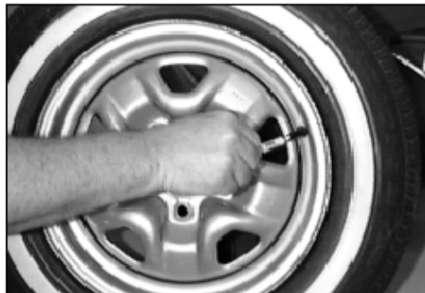
Figure 1 – Remove Valve Core to Deflate Tire
