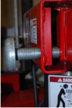
Adjust Swing Arm Adjusting Knob for proper distance from rim.
