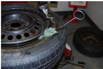
Lubricate rim and tire on both sides for easy removal and to prevent damage to tire and rim.
