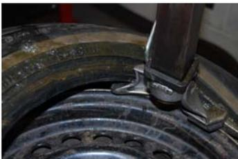
Position mounting head to rim position and rotate bottom bead to tight position around rim by depressing rotation pedal.
