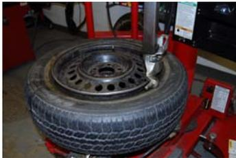
Full view of wheel and tire with head placement.
