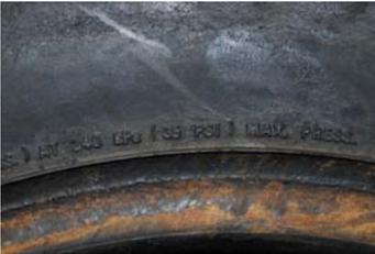
Inspect complete tire for damage and maximum tire pressure.
