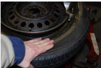
Repeat same step for top bead. Press bead into wheel well and slowly rotate tire until whole tire is over bead and onto rim by depressing rotation pedal.
