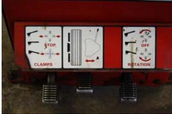
Repeat top bead step and press rotation pedal down and rotate bed counter clockwise lifting up on tire until top bead is removed from rim.
