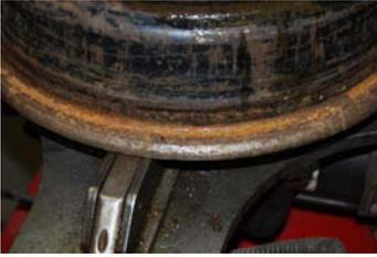
Inspect rim for rust, dents, and surface damage.
