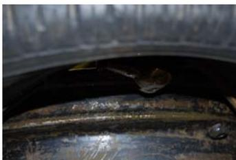
Underside view of lifting tool and bead when removing upper bead.
