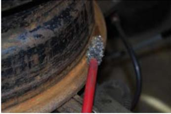
Clean all rust and debris from rim bead/flange. If surface is rough and/or pitted apply bead sealer to rim before installation. Make sure you are using goggles(dust mask if necessary).
