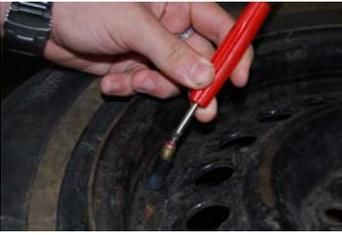
Remove valve core using core tool.
