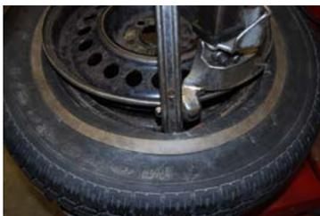
Position bead lifting tool over demount head and under top bead of tire.
