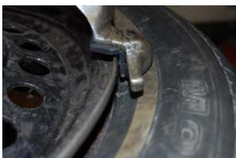
Position Slide/Demount Head to rim bead flange by pushing downward on slide.
