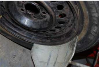
Position wheel between bead loosening shoe and front side of rim/tire.
