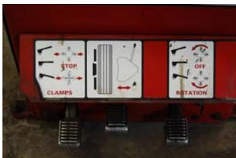
Press rotation pedal down and rotate table counter clockwise, lifting up on tire until top bead is removed from rim.
