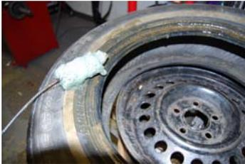
Lubricate both sides of tire with approved bead sealer before installation.
