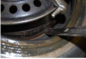
Using bead lifting tool grab lower bead and pull upward over demount head.
