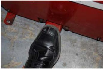
Depress inflation pedal while pulling up tire to make seal between rim and tire. Machine will cycle on and off to prevent continuous inflation. If tire does not inflate depress pedal further to engage bead seating application.
