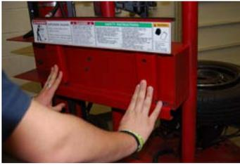
After tire has been released from rim clamp, position yourself behind inflation guard and begin to inflate tire to recommended pressure while monitoring pressure on gauge.
