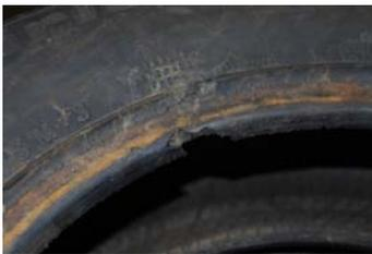
Check tire bead for cracks, tears and damage.
