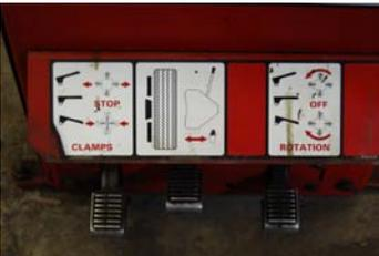
Press centre pedal until bead breaks from rim. Rotate wheel if not completely broken around tire.
