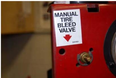
If tire pressure has exceeded recommended pressure, the manual tire bleed valve can be utilized to release pressure by pressing downward on valve.
