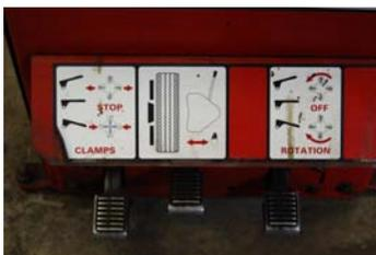
Remove rim clamp and have tire sit on table unsecured by depressing pedal before inflating tire to recommended pressure.
