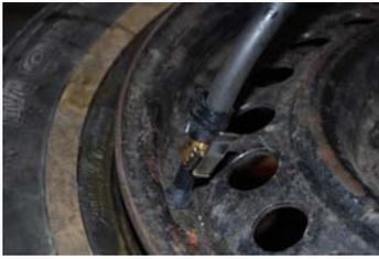
After tire is on rim properly attach air chuck to tire valve without valve core.
