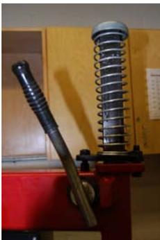
Push Vertical Slide Locking Handle away to allow for slide/demount head movement.
