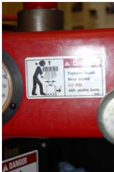
Observe maximum air pressure of **40 Psi** when seating bead to avoid **tire explosion and serious injury.**
