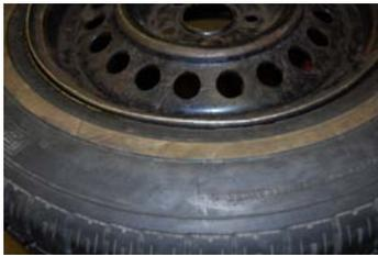
When tire begins to seal (hold air) on rim, stop and install valve core. **Do not continue to inflate tire and prevent tire explosion.**
